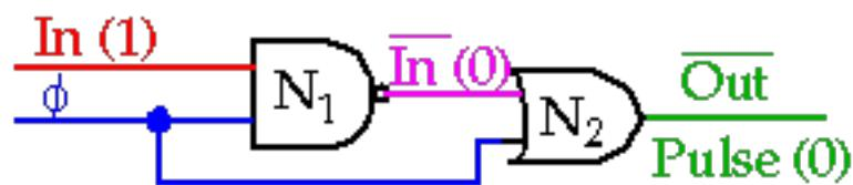
Results in a short low-going pulse at the output of  $N_2$  with length approximately equal to the propagation delay through  $N_1$ .
