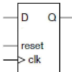
Edge triggered, synchronous reset, clock enable D flip-flop: C
