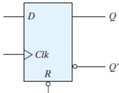
Edge triggered, asynchronous reset D flip-flop:
